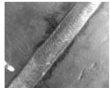
Figure 2. Close up of the orbital weld seam in the supermartensitic pipeline material.
