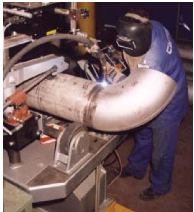
Figure 2. A complete ESAB solution for the mechanised TIG welding of stainless pipes.
