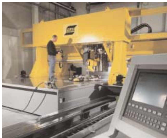
The FSW plant at DanStir, Denmark.
