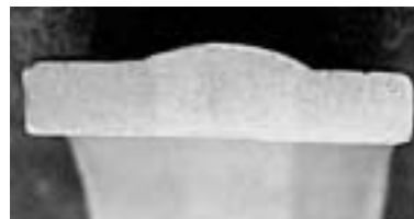
Figure 2. Weld appearance and macro of orbital weld.
