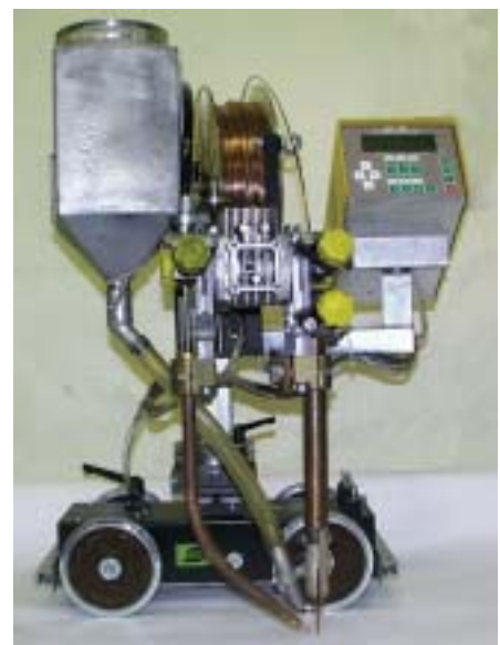
Figure 1. Submerged arc welding equipment (ESAB A6 Mastertrac) with Synergic Cold Wire kit.
